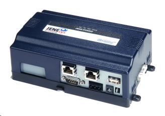
Modbus, oBIX and Internet standards. The AX Framework also includes integrated network management tools to support the design, configuration, installation and maintenance of interoperable networks.
